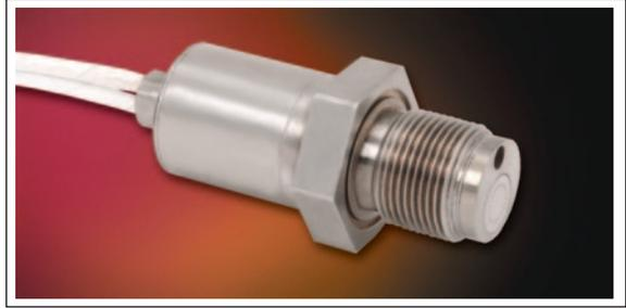
The XTEL-SD-625 Series are high temperature extremely rugged pressure transducers which are ideal for the measurement of flow instabilities and steady pressures in gas turbine combustors and compressors. The XTEL-SD-625 uses an innovative low-pass mechanical filter to enable the measurement of low-level dynamic pressures in high pressure environments with superior signal to noise ratios.
